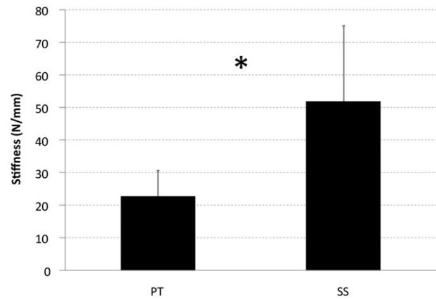
**FIGURE 5:** Mean stiffness (N/mm) for SS and PT repair techniques. The asterisk indicates a statistically significant difference between the 2 repair types. Standard deviation bars are shown.
