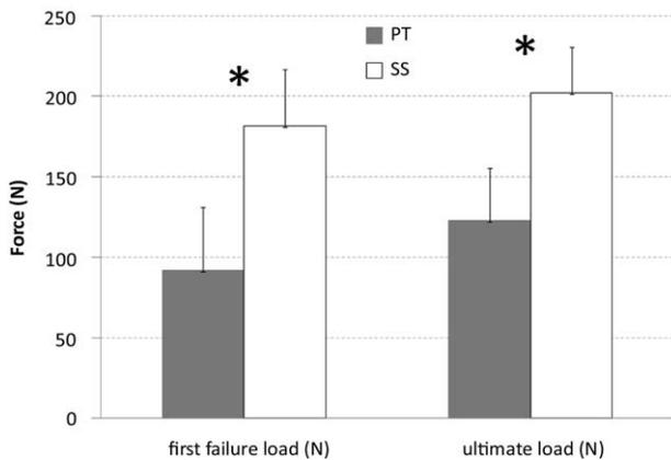
**FIGURE 4:** Mean first failure and ultimate loads (N) for SS and PT repair techniques. Asterisks indicate a statistically significant difference between the 2 repair types. Standard deviation bars are shown.
