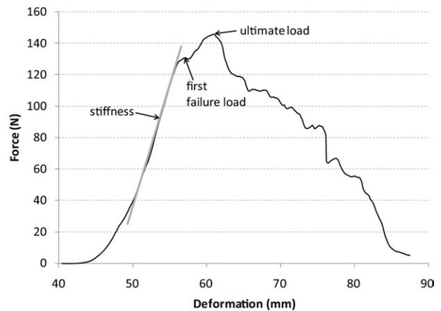
**FIGURE 2:** Representative force-deformation curve for a PT repair. Stiffness was calculated as the slope of the linear portion of the force-deformation curve.
