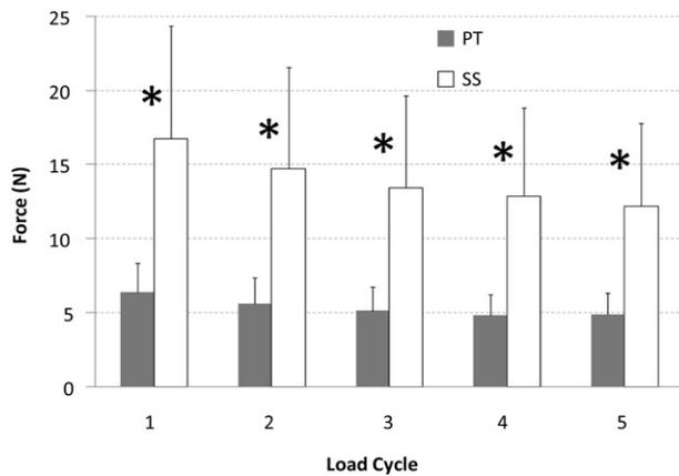
**FIGURE 3:** Mean load (N) reached at each the peak of each of the 5 conditioning cycles. A statistically significant difference (\*) was found between SS and PT repairs at each cycle. Standard deviation bars are shown.
